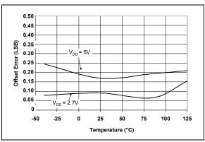
FIGURE 2-22: Offset Error vs. Temperature.
