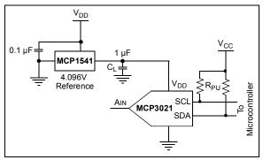
**FIGURE 6-7:** Stable Power and Reference Configuration.
