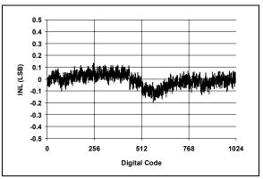
**FIGURE 2-6:** INL vs. Code (Representative Part,  $V_{DD} = 2.7V$ ).
