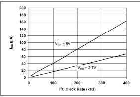
FIGURE 2-31: I<sub>DD</sub> (Conversion) vs. Clock Rate.
