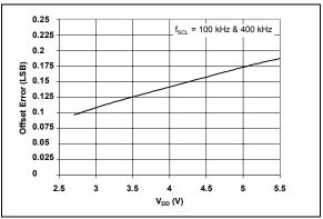
FIGURE 2-18: Offset Error vs. V<sub>DD</sub>.
