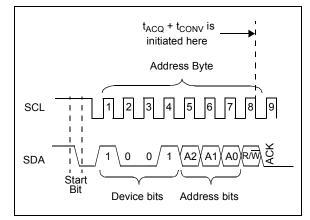
FIGURE 5-3: Address Byte.
