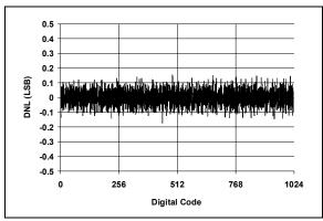
**FIGURE 2-16:** DNL vs. Code (Representative Part,  $V_{DD} = 2.7V$ ).
