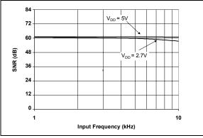
FIGURE 2-20: SNR vs. Input Frequency.
