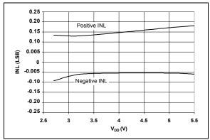
**FIGURE 2-2:** INL vs.  $V_{DD} - l^2 C$  Standard Mode ( $f_{SCL} = 100 \text{ kHz}$ ).
