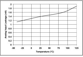
**FIGURE 2-38:** Analog Input Leakage vs. Temperature.
