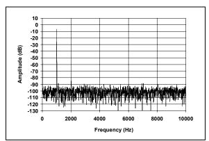
**FIGURE 2-27:** Spectrum Using I<sup>2</sup>C Fast Mode (Representative Part, 1 kHz Input Frequency).
