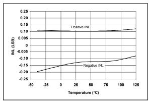
FIGURE 2-10: INL vs. Temperature  $(V_{DD} = 2.7V)$ .
