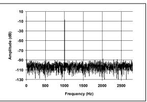
**FIGURE 2-29:** Spectrum Using I<sup>2</sup>C Standard Mode (Representative Part, 1 kHz Input Frequency).
