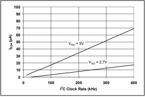
FIGURE 2-34: I<sub>DDA</sub> (Active Bus) vs. Clock Rate.
