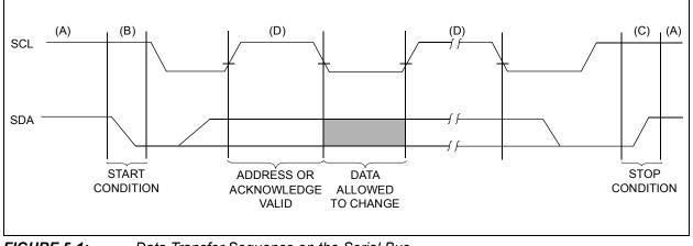
FIGURE 5-1: Data Transfer Sequence on the Serial Bus.
