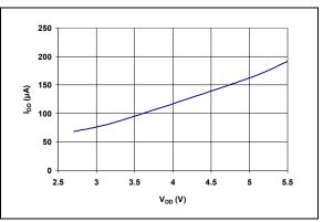
**FIGURE 2-30:**  $I_{DD}$  (Conversion) vs.  $V_{DD}$ .
