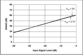
FIGURE 2-24: SINAD vs. Input Signal Level.
