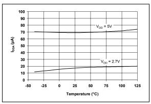
**FIGURE 2-35:** I<sub>DDA</sub> (Active Bus) vs. Temperature.
