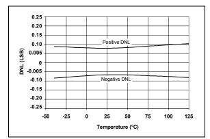
**FIGURE 2-17:** DNL vs. Temperature (V<sub>DD</sub> = 2.7V).
