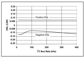
FIGURE 2-8: DNL vs. Clock Rate.
