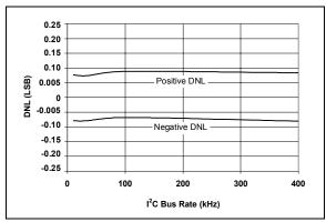
**FIGURE 2-11:** DNL vs. Clock Rate (V<sub>DD</sub> = 2.7V).
